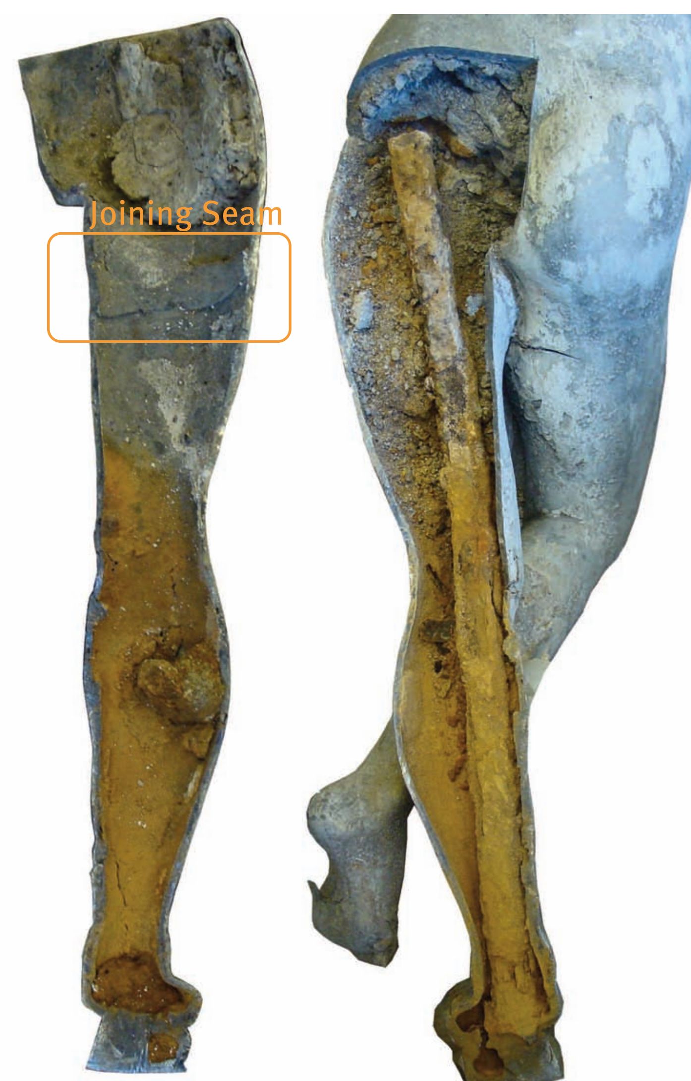
Fig. 5: The open left leg of the Dancer mainly without plaster core: the iron extends only up to the hip and is in a good condition. The thigh has a joining seam.
